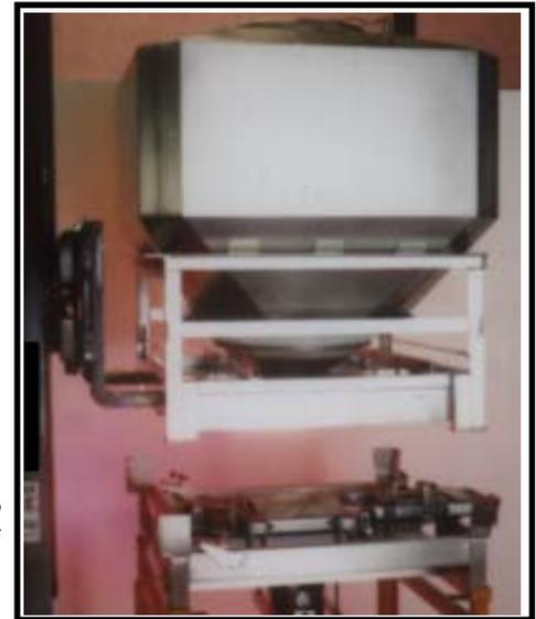
Application showing stainless steel Linkbin system, for use in hygienic fine chemicals manufacturing process.
